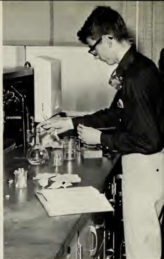
Measuring solutions in semi-microscopic qualitative analysis.
